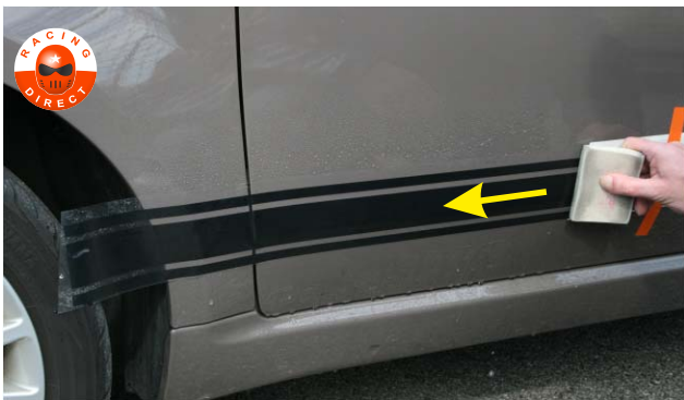
STAGE 8 - Press more time with the spatula to remove all the bubbles.
