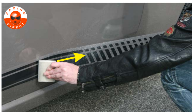
STAGE 12 - Paste the sticker and chasing water and bubbles with a spatula.
