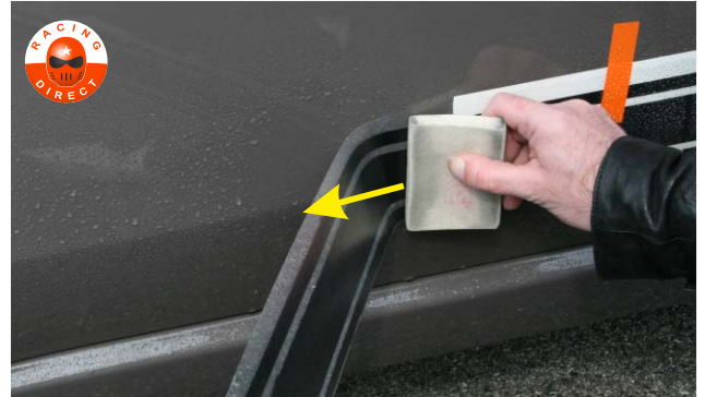
STAGE 7 - Paste the sticker and chasing water and bubbles with a spatula.
